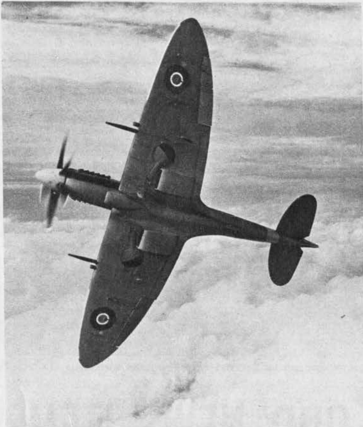
Spitfire XIV in this wing-over view shows the beautiful ellipse of its wing. Leading edge is slightly straighter than on the original model.
